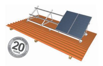
CompactGrid is a tilted mounting system for flat and pitched roofs which are east/ west facing. This system is specifically designed to distribute load evenly while spanning large distances between perlins. The Schletter DN rail series is used as a distribution rail below the triangular supports, which hold the array in place.
