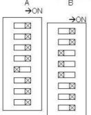
10.5V low alarm on 11.5V alarm off 15.5V high
